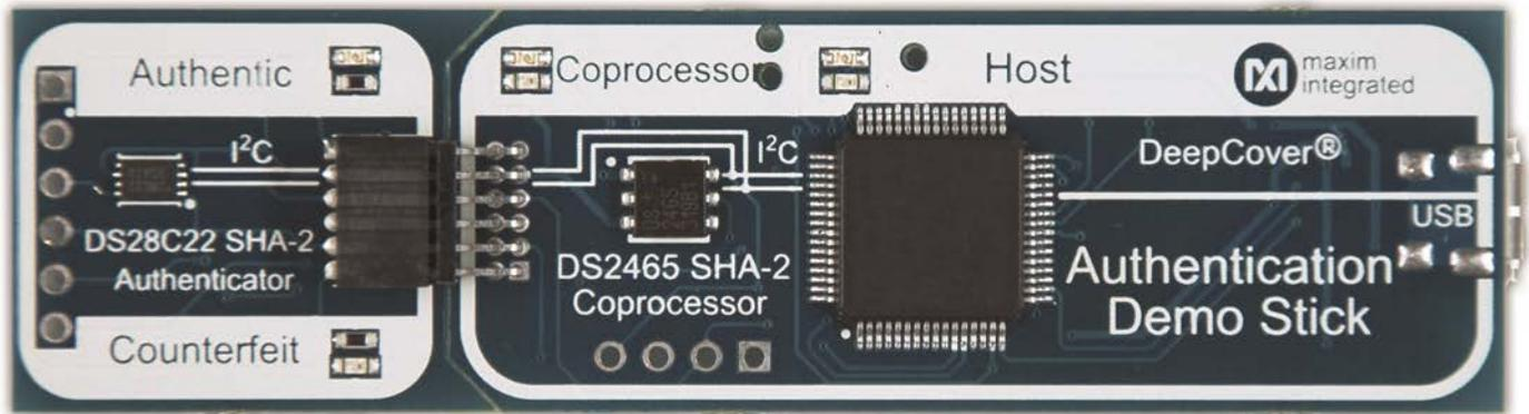
The DS28C22 Authentication Demo Stick comprises a host board, a slave DUT board, and a USB cable. The host board contains a MAXQ622 power microcontroller and a DS2465 secure coprocessor. The microcontroller communicates over the I<sup>2</sup>C interface to the DS2465 and the DS28C22 slave. On one side of the slave DUT board is an authentic DS28C22 IC. The reverse side contains an unauthentic DS28C22 IC. The USB connection is used for power only.
