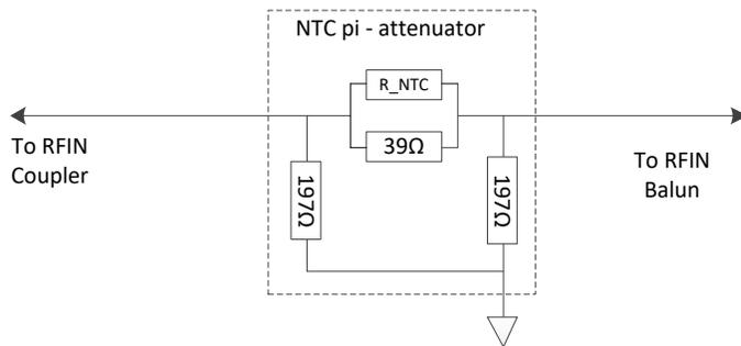
Figure 7. NTC attenuator in the RF input path.
