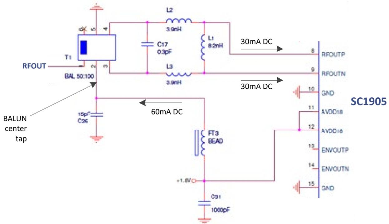
Figure 8. RFOUT BALUN, matching network and decoupling.
