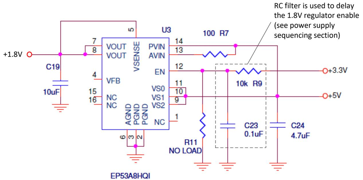
Figure 20. 5V to 1.8V switching regulator used in the SC1905 EV kit.
