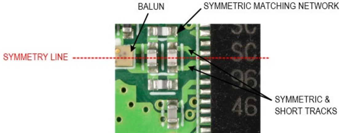
Figure 6. Balun + differential matching network.
