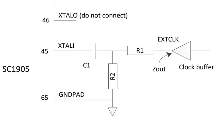
Figure 21. External clock diagram.
