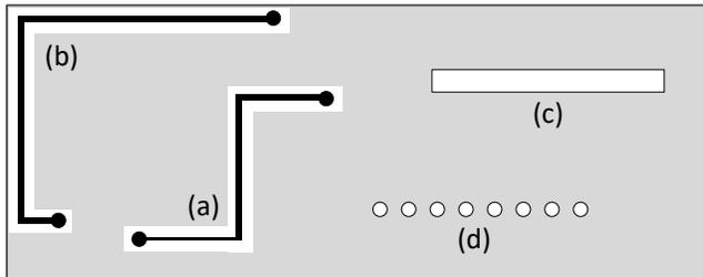
(a) Poor: trace cuts ground plane and prevents direct returns
