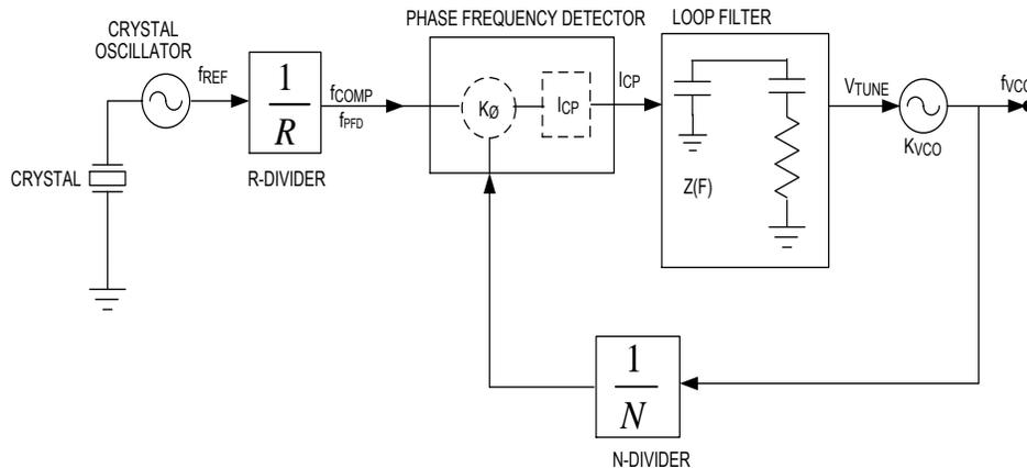
Figure 1. Block diagram of a typical PLL.
