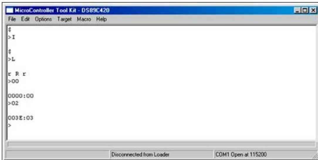
Figure 9. Screen shows the steps to erase the MAXQ7665's flash memory.
