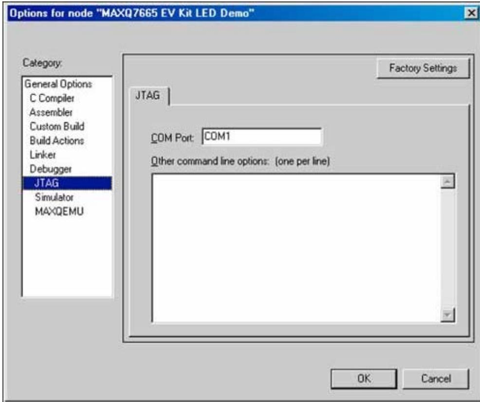
Figure 3. Communication between the IAR toolset and the MAXQ7665 is set up through the JTAG interface.
