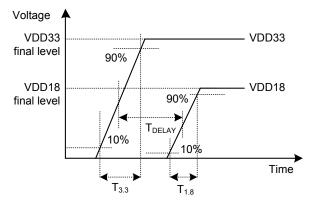
Figure 18. VDD18 and VDD33 power-on timing sequence.
