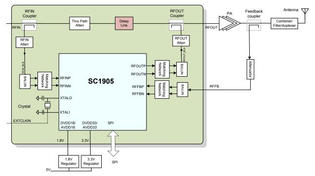
Figure 2. SC1905 reference design block diagram.
