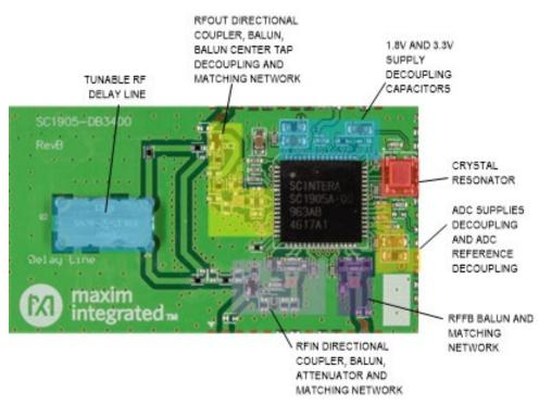
Figure 12. SC1905 reference board floor plan.
