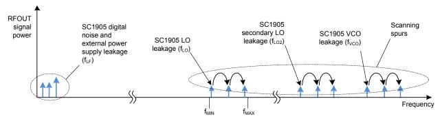
Figure 10. SC1905 spurious content (CAL mode).
