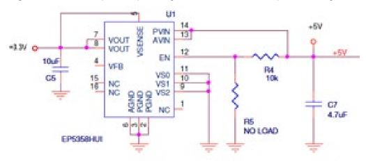
Figure 19. 5V to 3.3V switching regulator.
