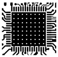
Figure 14. Via array under SC1905 ground paddle.
