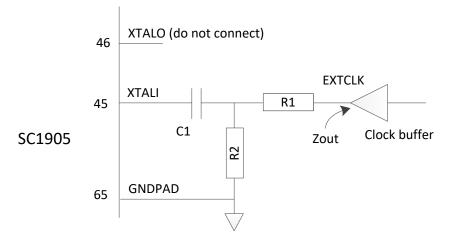
Figure 21. External clock diagram.
