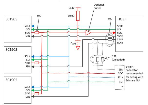
Figure 23. Host SPI connection for multiple SC1905 applications.
