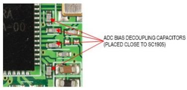
Figure 11. ADC decoupling capacitors.
