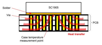
Figure 17. PCB fabrication layer stack.
