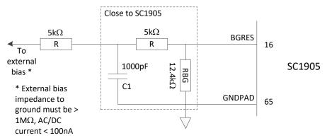
Figure 22. External bias circuit using the SC1905 bandgap voltage.
