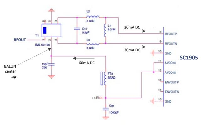
Figure 8. RFOUT BALUN, matching network and decoupling.
