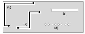
(a) Poor: trace cuts ground plane and prevents direct returns
