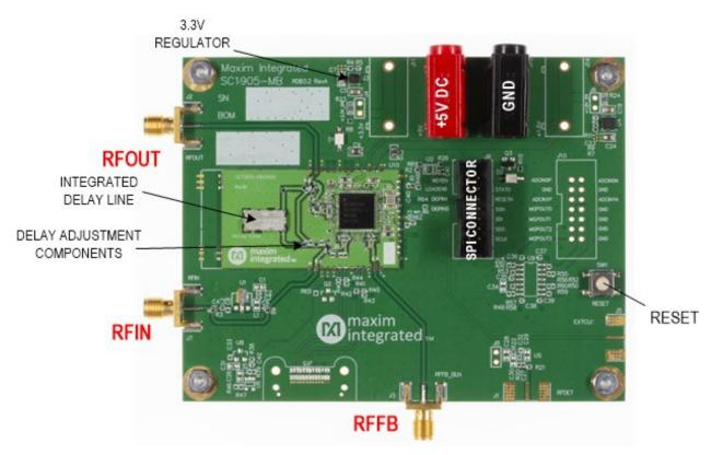
Figure 4. SC1905 reference board and motherboard.
