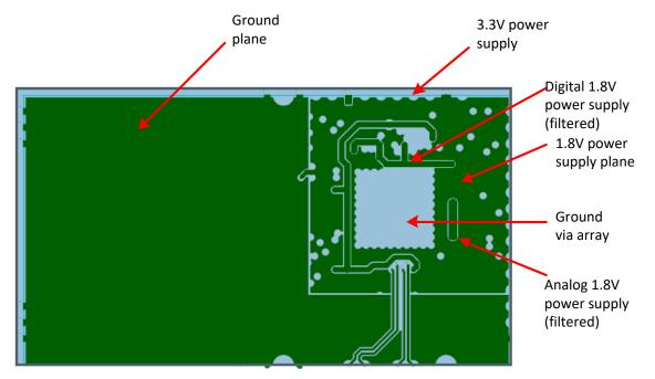
Figure 16. Layer 3, power supply distribution.
