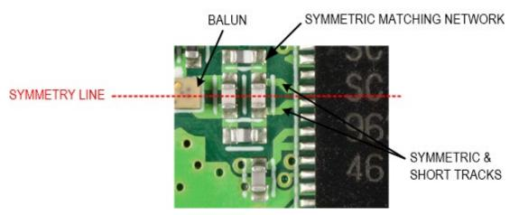
Figure 6. Balun + differential matching network.
