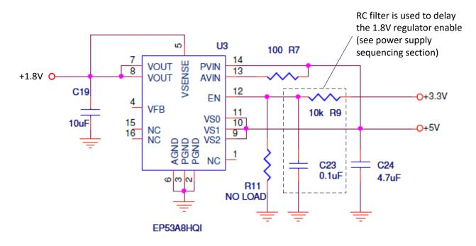
Figure 20. 5V to 1.8V switching regulator used in the SC1905 EV kit.
