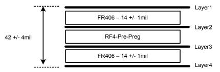
Figure 13. PCB fabrication layer stack.
