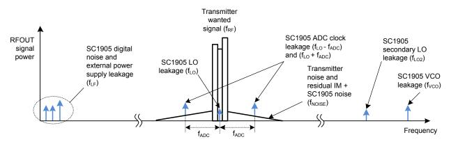
Figure 9. SC1905 spurious content (TRACK/FSA mode).
