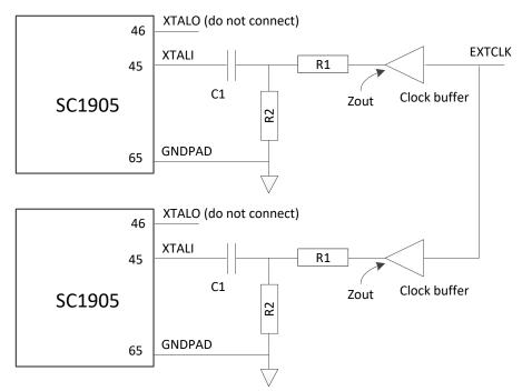
Figure 25. External clock diagram for multiple SC1905 applications.
