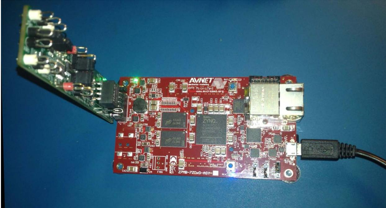
Figure 4. MAXREFDES5# Installed in J5 Connector
