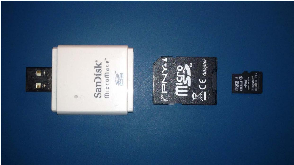
Figure 1. USB-SD, SD-Micro-SD, and Micro-SD Card
