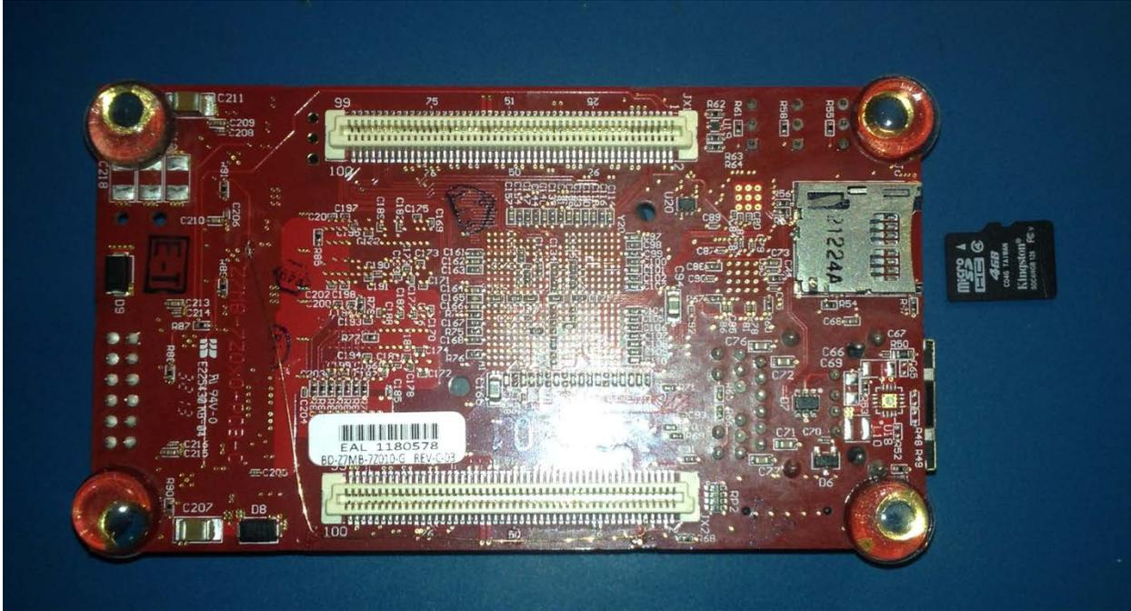
Figure 2. MicroZed SD Card Slot and Micro-SD Card
