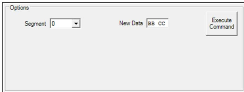
The screenshot shows a dialog box titled "Options" for the Write Memory command, specifically for general-purpose writing. It contains a dropdown menu for "Segment" with the value "0" and a text input field for "New Data" containing the hex digits "BB CC". To the right of these fields is a button labeled "Execute Command".
