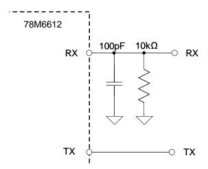
Figure 15: Connections for the RX Pin
