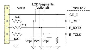
Figure 11: ICE Pin Used to Drive LCD Segments
