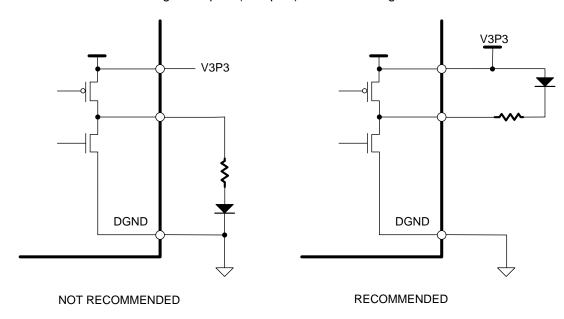
Figure 12: Connecting an External Load to a Digital Output
