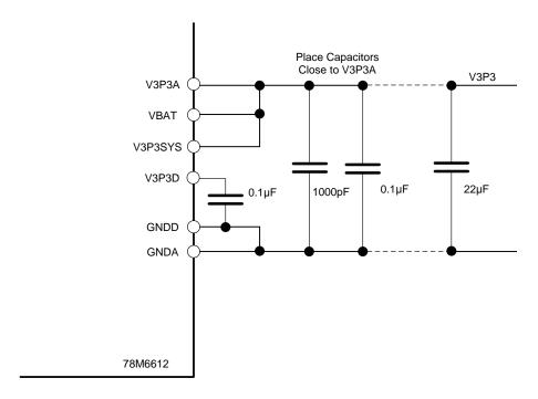
Figure 2: Power Supply Decoupling
