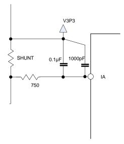
Figure 4: Shunt Connections and Filtering
