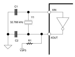
Figure 23: Crystal Oscillator with Pull-up to Reduce Startup Time
