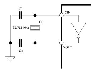
Figure 19: 78M6612 Crystal Oscillator Connection
