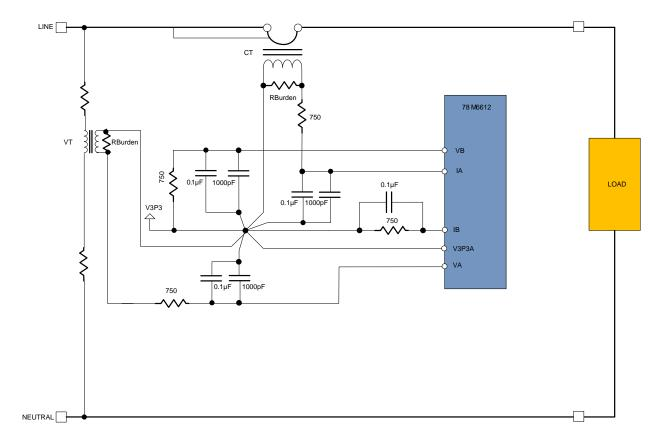
Figure 7: Basic Connection Diagram of a CT and VT Based System
