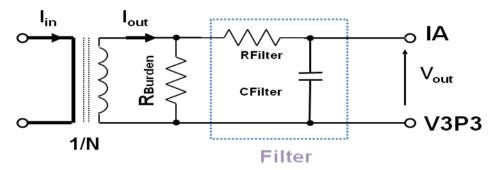
Figure 5: Current Transformer (CT) Basic Connections
