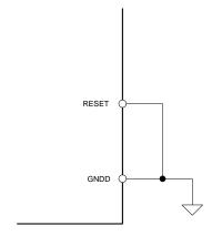
Figure 9: Connection for Unused Reset Pin
