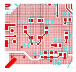
Figure 20: Crystal Y1 and Capacitors C7/C9
