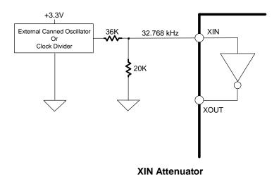
Figure 25: 78M6612 with External Canned Oscillator
