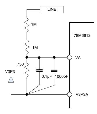
Figure 3: Input Voltage Divider and Filtering
