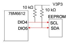
Figure 13: I<sup>2</sup>C EEPROM Connection
