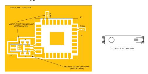
Figure 22: Crystal Oscillator Components on the Same Side
