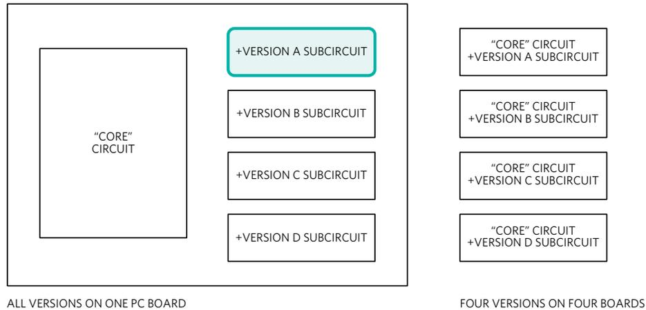
Figure 1. An all-encompassing circuit (1a, left) integrates all anticipated version needs into a single circuit; a tailored design (1b, right) breaks out functions designed for each required end application.
