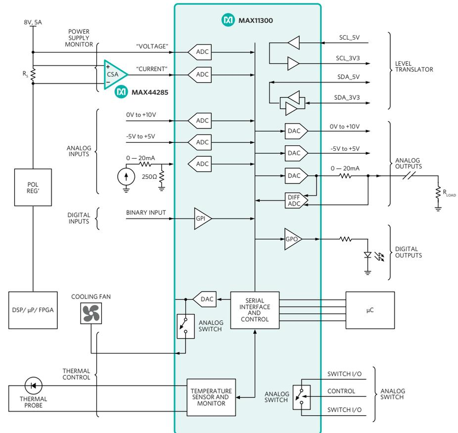
Figure 3. Control and monitoring with the MAX11300.
