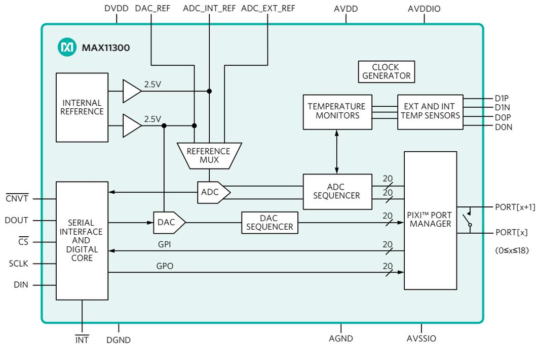
Figure 2. The PIXI programmable, mixed-signal IO allows 20 used-defined, programmable ADC, DAC, or GPIO functionality.
