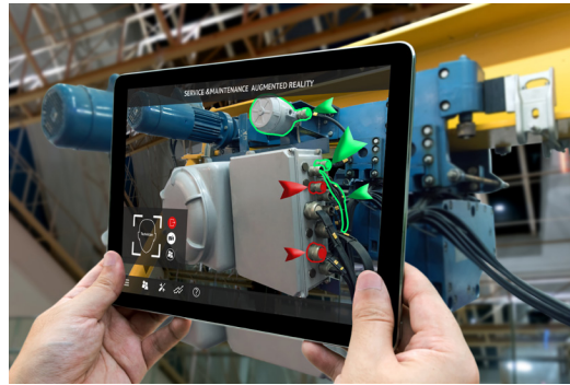
Figure 4. Service Maintenance Aided by a Hand-Held Tablet Equipped with AR
