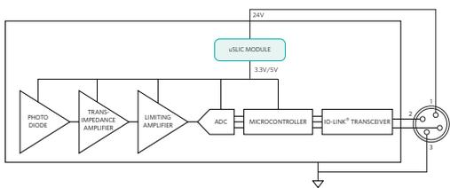
**Figure 8.** Typical optical proximity sensor system block diagram
