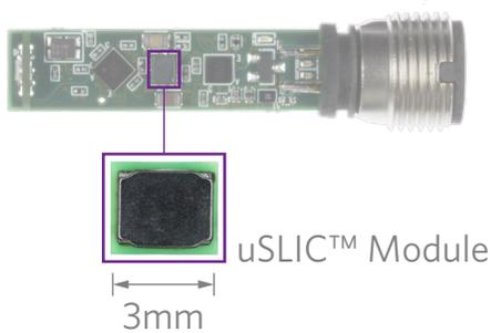
**Figure 7.** MAXM17532 in a tiny proximity sensor
