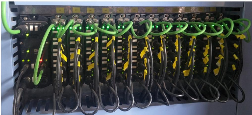
GSEE-TECH's 4-/8-channel analog input block, designed for use with Maxim's MAX11270, is very small and low power, has self-configurable current and voltage signals, and features 16-bit high precision, wide operation temperature, and low temperature drift.
