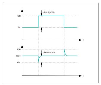
Figure 9. Output load step response.
