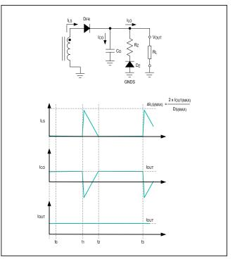
Figure 8. Secondary-side circuit and currents.
