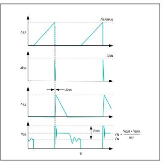
Figure 6. RCD snubber circuit waveforms.
