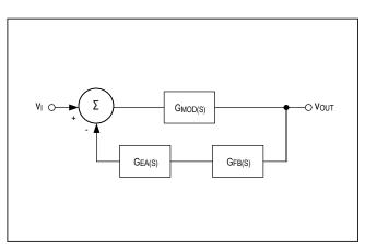
Figure 10. Simplified model of control loop.
