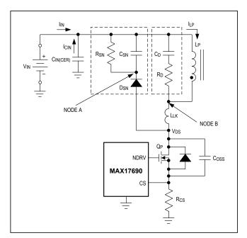
Figure 5. RCD snubber circuit.
