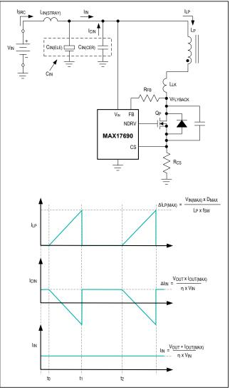
Figure 7. Primary-side circuit and currents.
