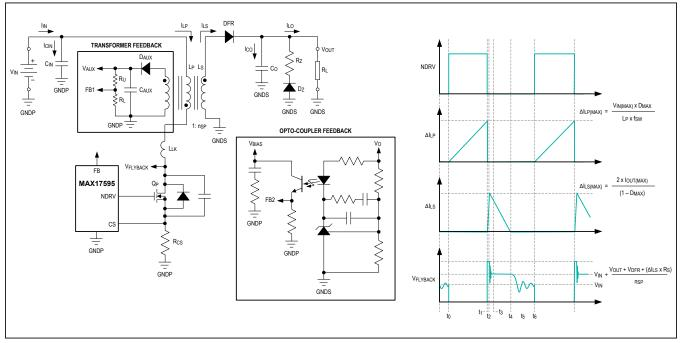
Figure 2. Isolated flyback converter topology with typical waveforms.
