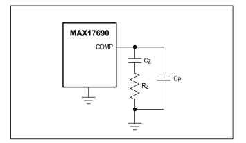
Figure 11. Type II compensation for OTA.
