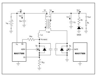
Figure 4. Simplified no-opto flyback schematic with synchronous rectification.
