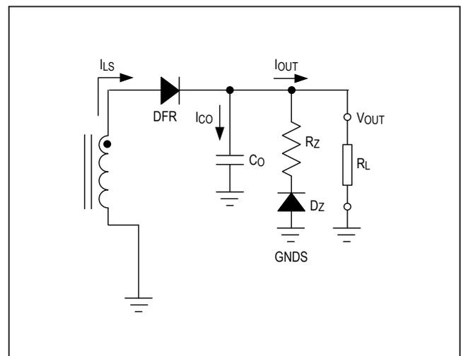
Figure 7. Simplified no-opto flyback schematic with Schottky diode.
