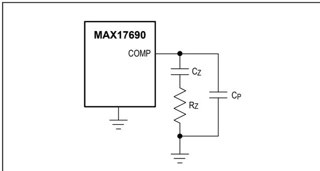
Figure 14. Type II compensation for OTA.
