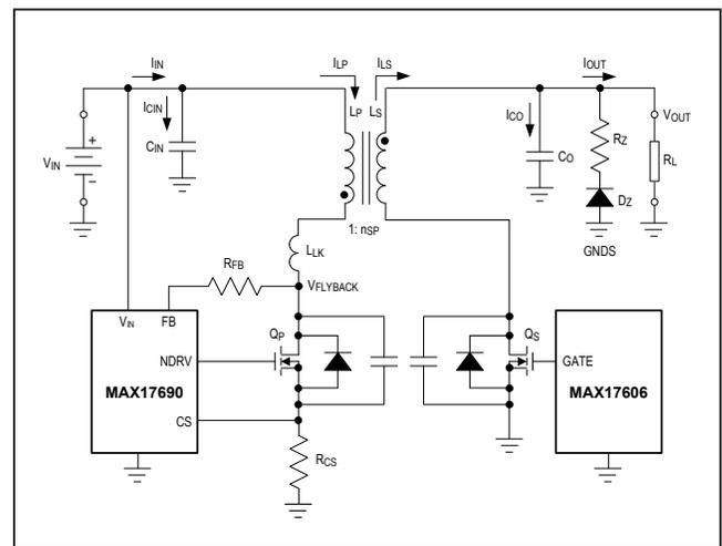
Figure 4. Simplified no-opto flyback schematic with synchronous rectification.
