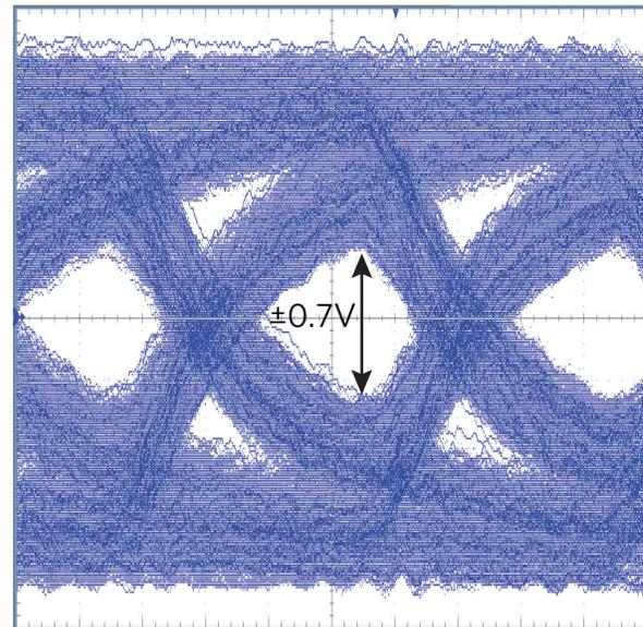
Figure 4. MAX22500E Operating at 50Mbps Over 100m Cat5e (Scale at 5ns/div)
