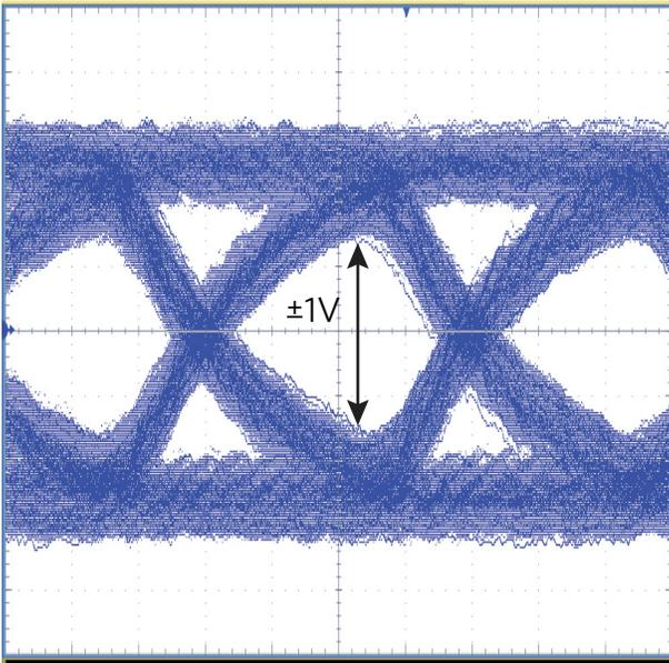
Figure 5. MAX22500E Operating at 50Mbps Over 100m Cat5e with Pre-emphasis Enabled (Scale at 5ns/div)
