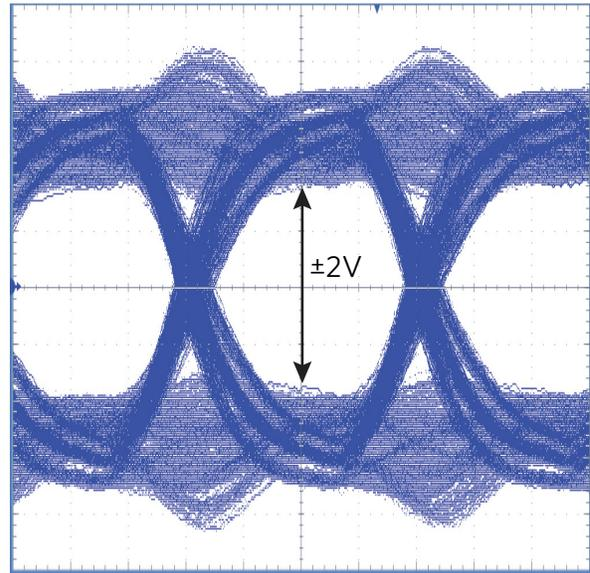
Figure 3. MAX22500E Operating at 100Mbps Over 10m Cat5e (Scale of 2.5ns/div)
