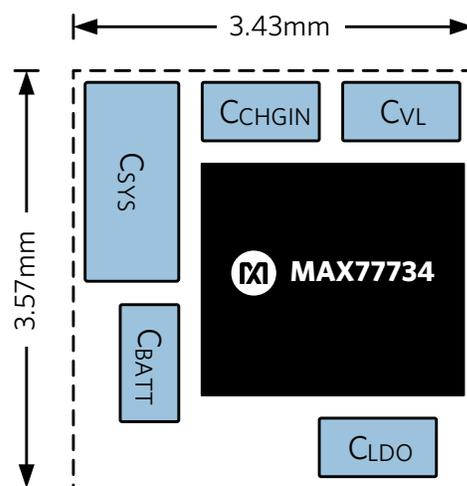
Figure 6. Integrated Charger and LDO Footprint (12.24mm<sup>2</sup>) with MAX77734
