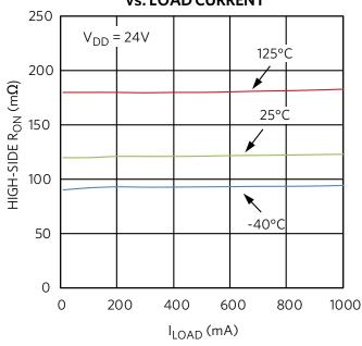
Figure 3. MAX14914 On-Resistance vs. Load
