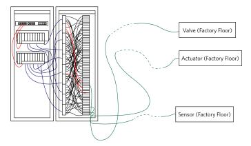
Figure 1. Wired Marshalling
