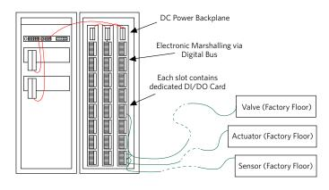
Figure 2. Electronic Marshalling
