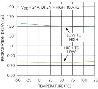
Figure 4. MAX14914 Propagation Delay in DI Mode
