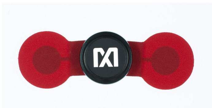
Figure 3. The MAX-ECG-MONITOR Evaluation and Development Platform
