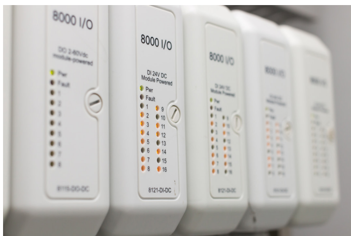
Figure 1. Programmable Logic Controller IO Module
