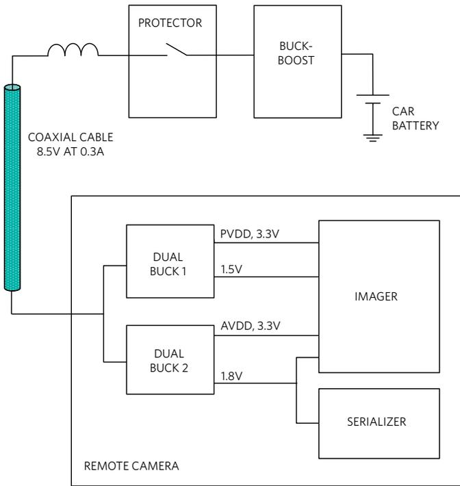
Figure 3. Remote Camera Single-Channel Detail
