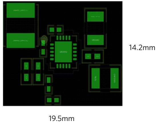
Figure 7. Buck-Boost Converter PCB Area (277mm<sup>2</sup>)
