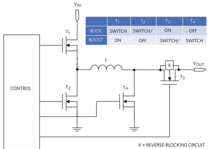
Figure 4. Buck-Boost Power Train Architecture and Operation Table
