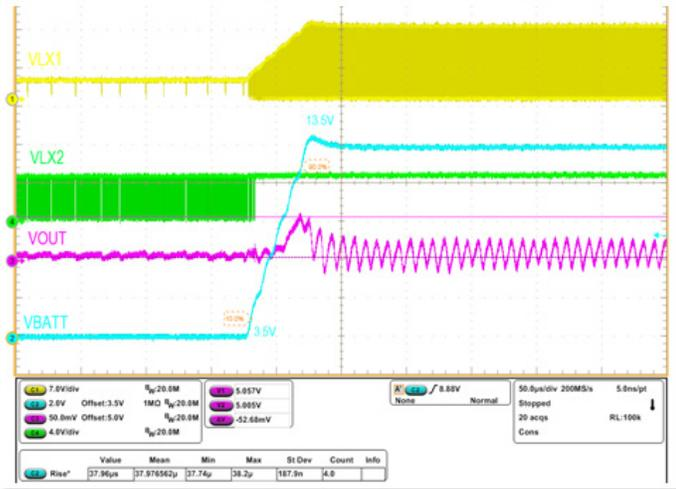
Figure 5. Positive Line-Transient Response
