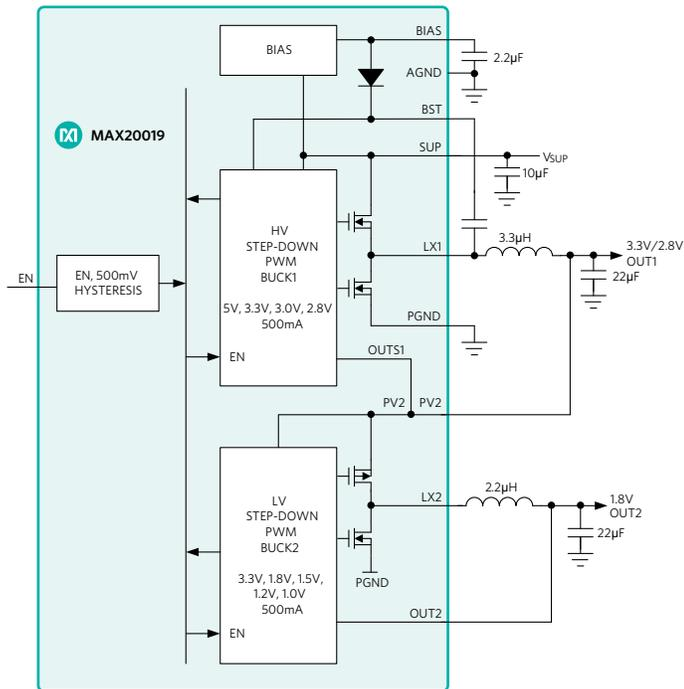
Figure 9. Dual Buck Converter Cascade
