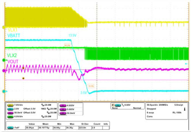
Figure 6. Negative Line-Transient Response
