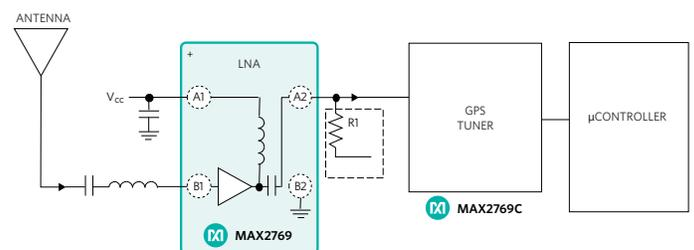
Figure 2. GPS Receiver Front-End Circuitry
