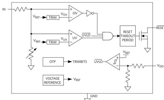
Figure 6. MAX16132  $\mu P$  Supervisor Block Diagram
