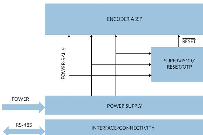
Figure 4. Encoder ASSP Power Rails Control
