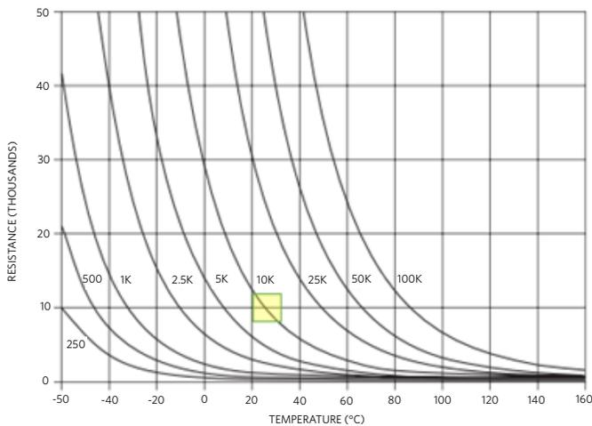
Figure 4. Resistance-Temperature Curves for Nine Common Thermistors
