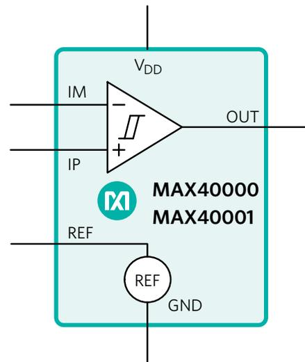
Figure 5. MAX40000/MAX40001 Functional Diagram
