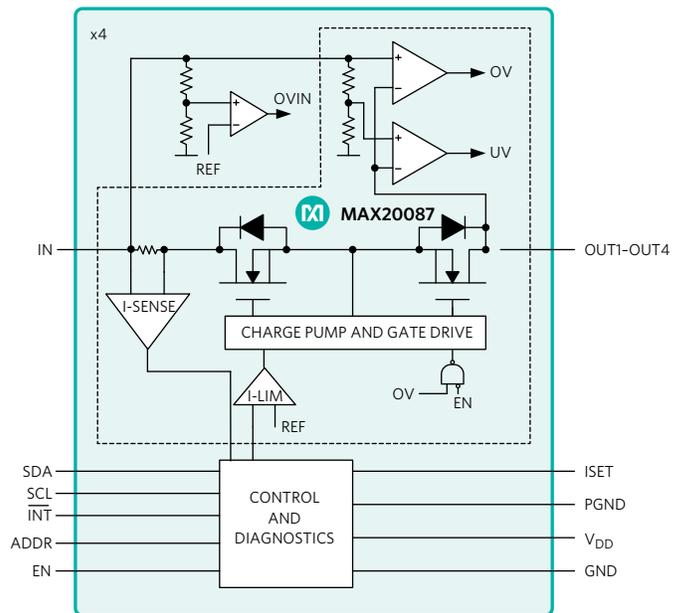
Figure 8. Input Current and Voltage Protection
