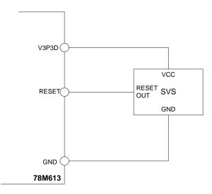
**Figure 9: Reset Generator Connection**
