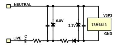
Figure 15: Simple Circuit Design for Low-Power Applications
