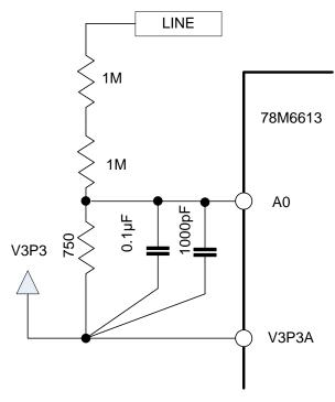
Figure 3: Input Voltage Divider and Filtering
