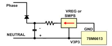
Figure 17: High Efficiency for Higher Power Applications
