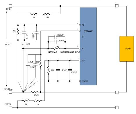
Figure 1: Basic Connection Diagram on Shunt-Based Systems
