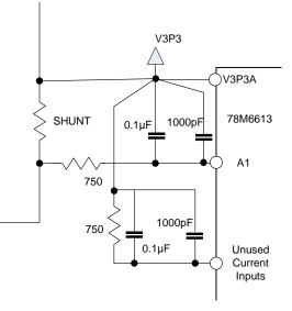
Figure 4: Shunt Connections and Filtering
