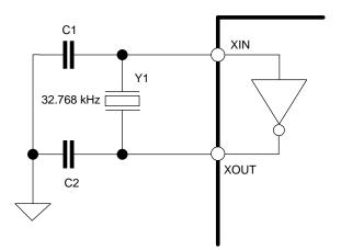
Figure 18: 78M6613 Crystal Oscillator Connection
