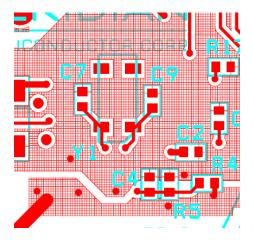
Figure 19: Crystal Y1 and Capacitors C7/C9
