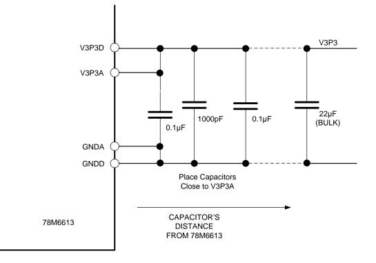
Figure 2: Power Supply Decoupling
