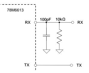
Figure 14: Connections for the RX Pin
