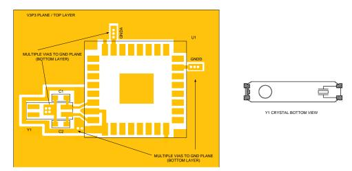
Figure 21: Crystal Oscillator Components on the Same Side
