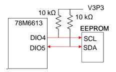
Figure 12: I<sup>2</sup>C EEPROM Connection
