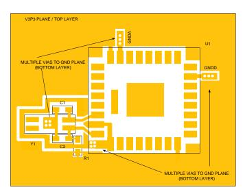
Figure 23: Example of Layout of Crystal Oscillator with Pull-up Resistor
